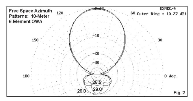
The antenna pattern itself is a model of good behavior, with no undesirable side or rear lobes. Note in **Fig. 2** the change in the shape of the rearward lobe across the band, which is a normal progression for well-behaved antennas of this type.
