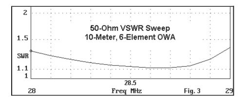
As a high-performance 10-meter antenna covering all of the first MHz of the band, the 24' 6-element OWA is a worthy monoband competitor with other designs for the band.
